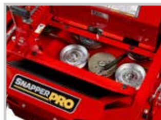
Quick removal of the floor pan provides easy access to the top of the deck when maintenance is needed.
