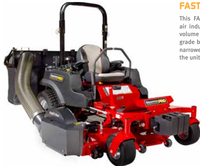
S200xt with FAST-Vac and a triple bag collection system. FAST-Vac Blower — Length: 36.8" Height: 20.2" Width 15.2"
