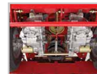
Self-contained dual hydro transmissions are individually fan cooled and filtered.
