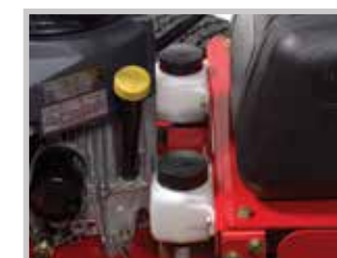
Dual hydro fluid reservoirs protect each hydro system from cross contamination.
